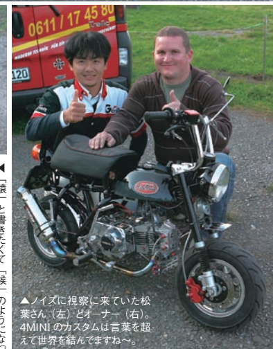
A.Komandriow (33 / Germany) Monkey (HONDA). This is the vehicle which Mr. Matsuba of G craft who is on study visit from Japan likes the most. It is unusual to remodel the Z50A which has high scarcity value into the disk brake, and used a lot of Japanese parts and the rare bottom case.
